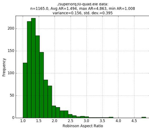
Figure 2: A quad mesh and the resulting histogram plot showing Robinson's aspect ratio distribution.
