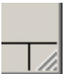
A palette group window without this size box in the lower-right corner cannot be resized.
