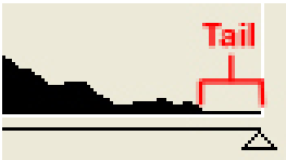
Some histograms have tail-like pixels at the black and white ends of the histogram. These indicate that few pixels have those brightnesses. Many people like to drag the sliders past these tails to force them to pure white or black.
