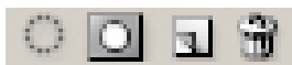
The Channels palette buttons include (from left to right) Load channel as selection, Save selection as channel, Create new channel, and Delete current channel.
